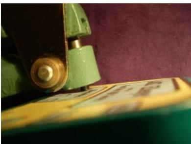
Nestle the center punch dimple onto the point of the punch and squeeze. It's as simple as that.
